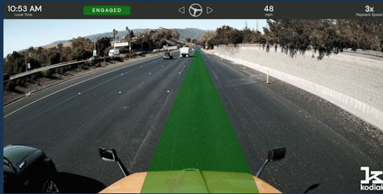
Weak lane markings
