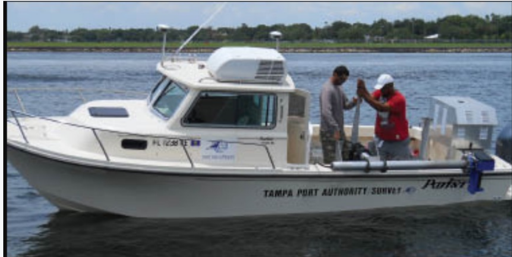
Tampa Port Authority surveyors prepare to lower their multibeam echo sounder into the water.
