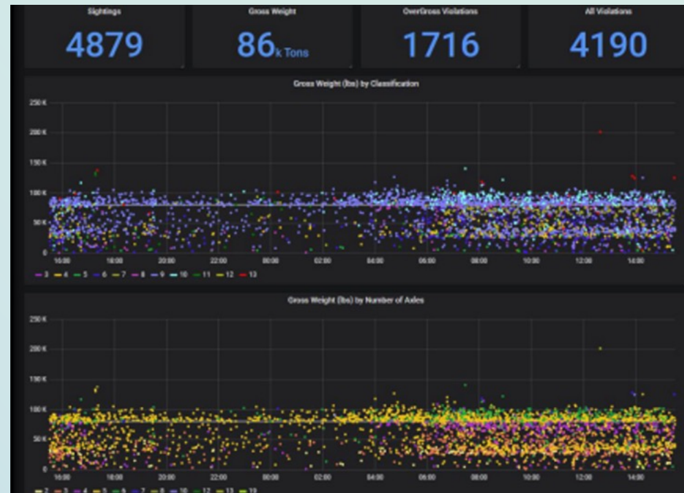
24-HR Snapshot of FOX Data: upper section provides overview gross weight by classification and the lower portion shows gross weight by number of axles.
